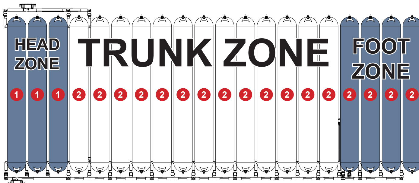
Fig. Structure of the 20 mattress cells
