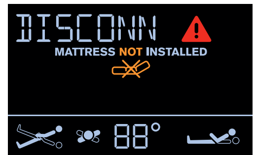
Afb. PUMP DISCONNECTED (POMP LOSGE- KOPPELD)
