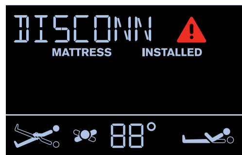
Fig. DISCONNECTED AIR PIPES
