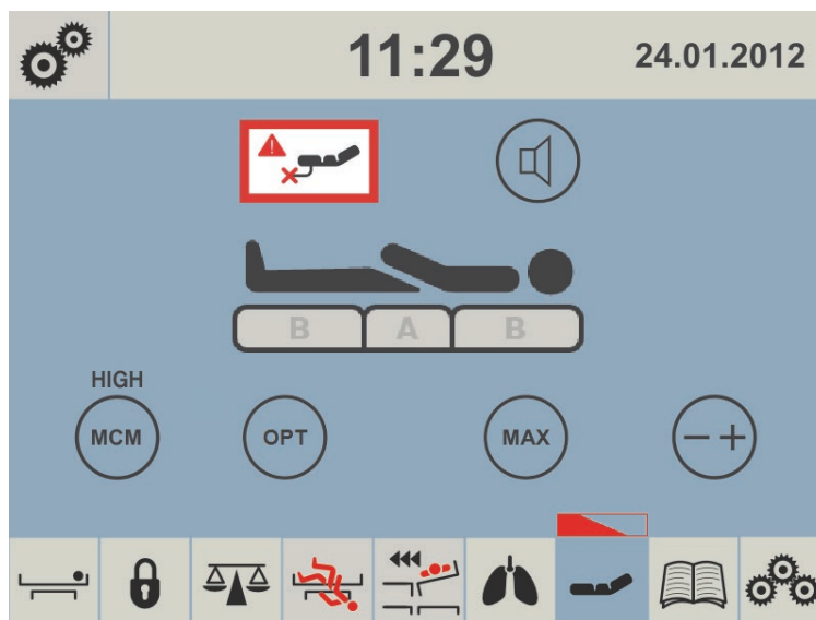
Fig. Alert – Disconnected Air Pipes
