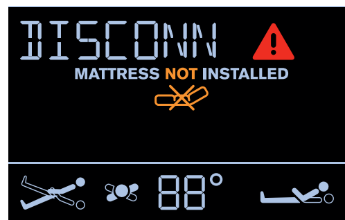
Fig. PUMP DISCONNECTED
