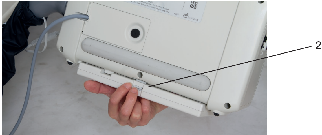
Fig. Removing the accumulator pack
