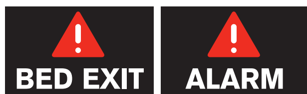
Fig. Visual signalisation of Bed Exit Alarm (alternation of the two inscriptions)
