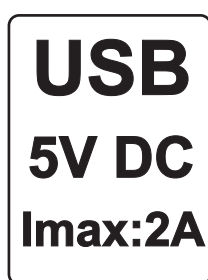
Fig. USB label with electric specifications
