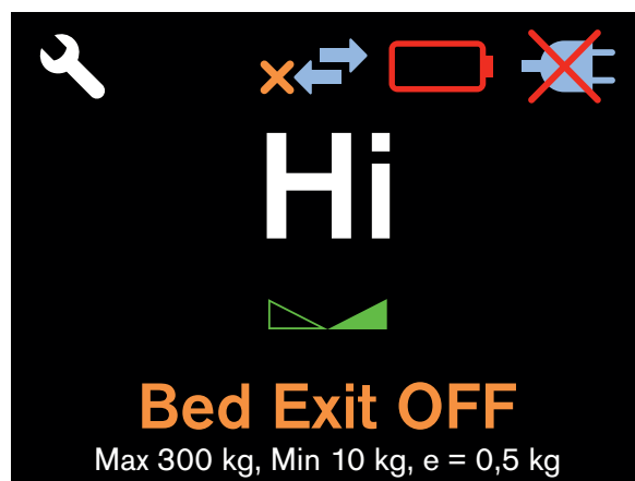
Fig. Mattress support platform is overloaded (pop-up screen)
